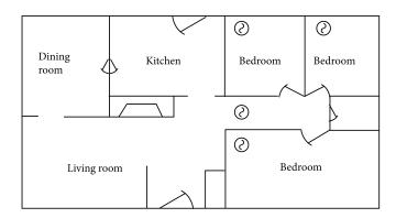
Wall-mounted smoke alarms should be installed so that the top of the alarm is not more than 12 inches (30.5 centimeters) from the ceiling.
