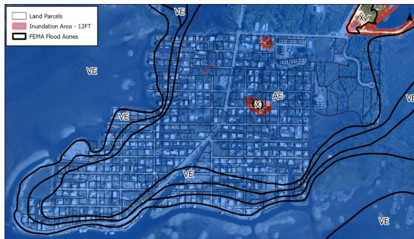
Parcel-level analysis correlating to FEMA zone designations with observed storm damage by event.
