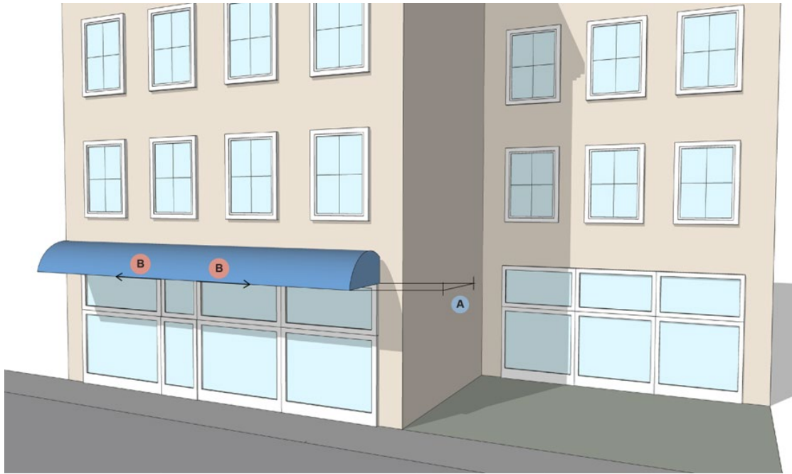
Figure 225-20-B: Front façade recessing
