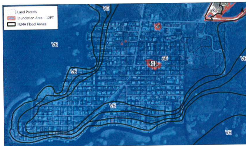
Parcel-level analysis correlating to FEMA zone designations with observed storm damage by event.
