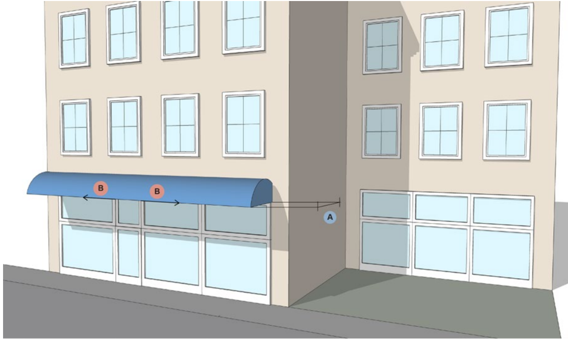
Figure 225-20-B: Front façade recessing
